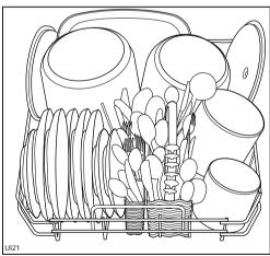
Cutlery should be placed in the removable cutlery basket with the handles facing downwards. If the handles protrude from the bottom of the basket, obstructing the lower spray arm, load the cutlery with the handles facing upward.
